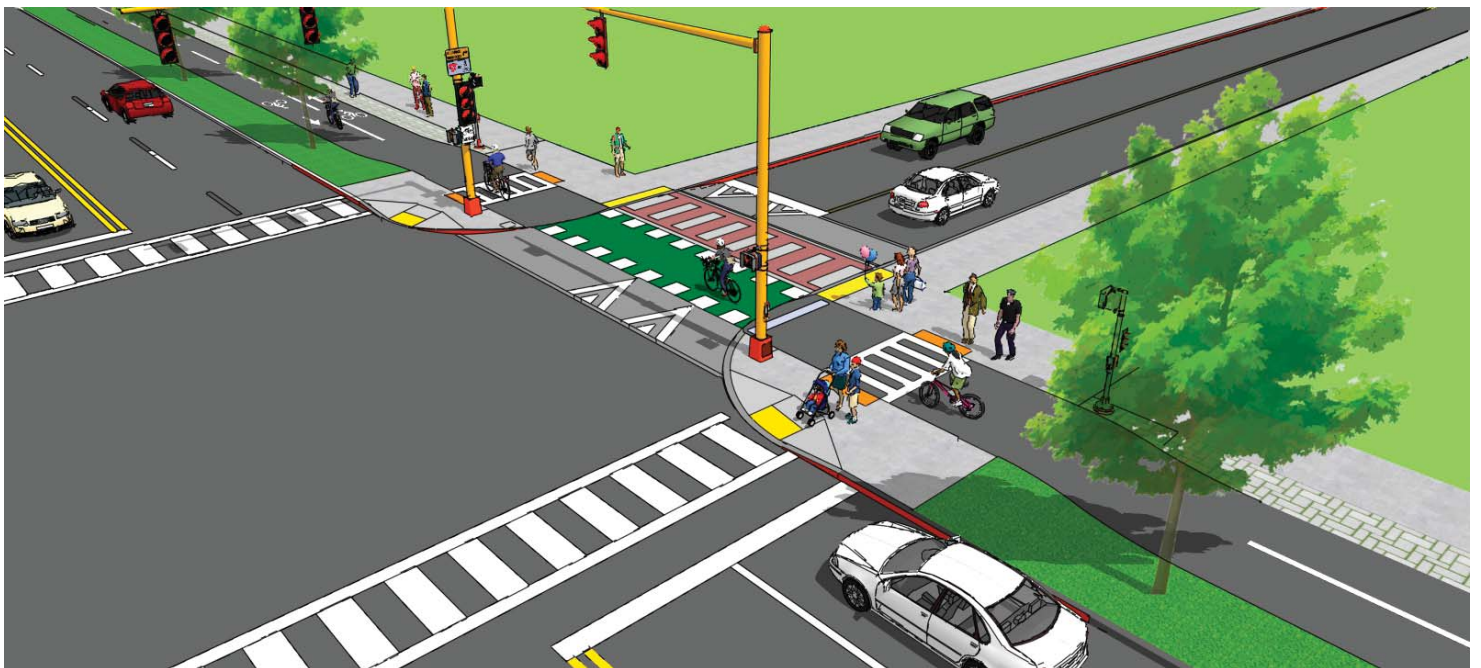
Protected intersection and driveway crossings help minimize bicyclist exposure to motorized traffic.
