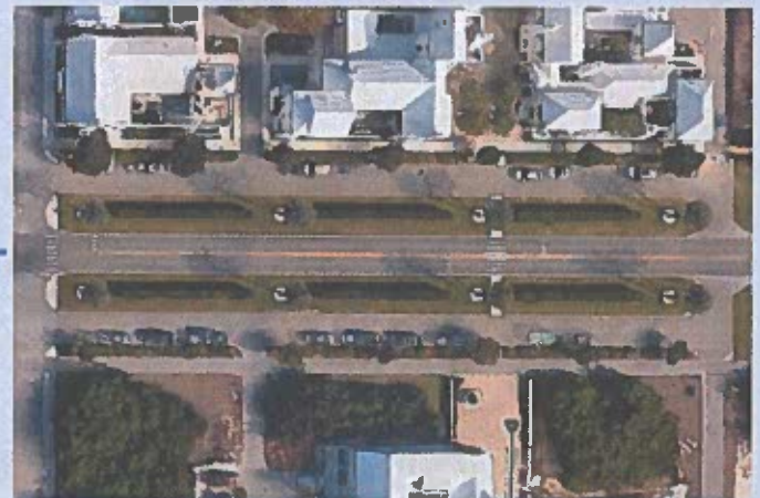
Example: A tree lined county road in Aly's Beach, FL. The slip lanes provide additional parking, a bike path, and keep local traffic and highway thru-traffic separate. (GoogleMaps)
