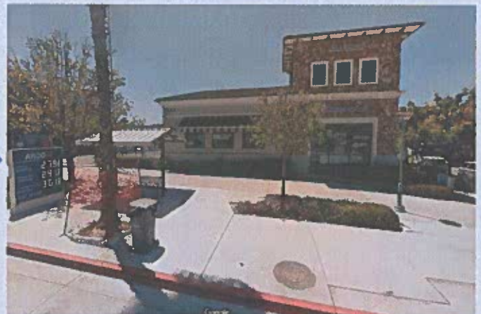
Form Based Code: An Arco gas station in Chula Vista, CA. The mini-market and a small gas sign front the street, while the pumps are located in the rear of the lot.
