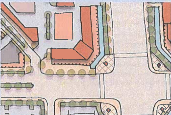
Plan: Existing gas station on the corner of Bonita Beach Road/Tamiami Trail is retrofitted with a corner store liner.
